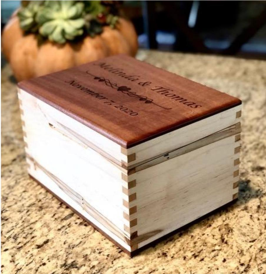
I built a wedding keepsake box for the daughter of good friends. The top and bottom is Sapele and the sides are Western Maple. I used a homemade box joint jig on the table saw for the joinery. The corners are a four-corner match. The laser lettering was done by Jason at the Woodshed.
