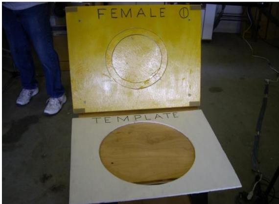
Once again inlay routing results in one piece completely contained by the other as shown in the picture left. Bushings, collets and templates of any shape, any size may be used in this process.
