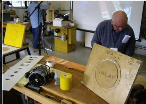
made with a straight bit in the router. The technique for cutting with the router as described in the above picture is “inside cut clockwise”, “outside cut counterclockwise.” Howard’s formula for bushing size as described above is “Small bushing Diameter size plus 2 times bit diameter size equals Large Bushing Diameter. This formula is essential to understanding and executing inner and outer pattern cuts using the router.
